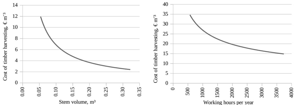
Fig. 2. Stem volume and harvester utilization rate impact on timber harvesting costs
